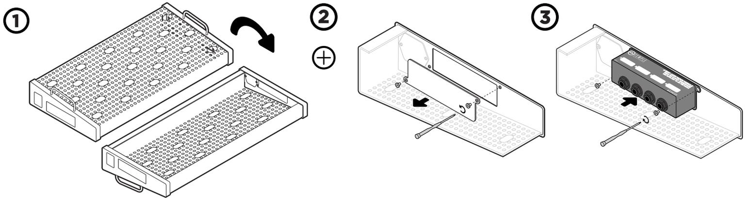
The 4X MOD mounts in the Modular Endpanel of your Templeboard and allows you to route 1/4" inputs and outputs through the side of your board.
