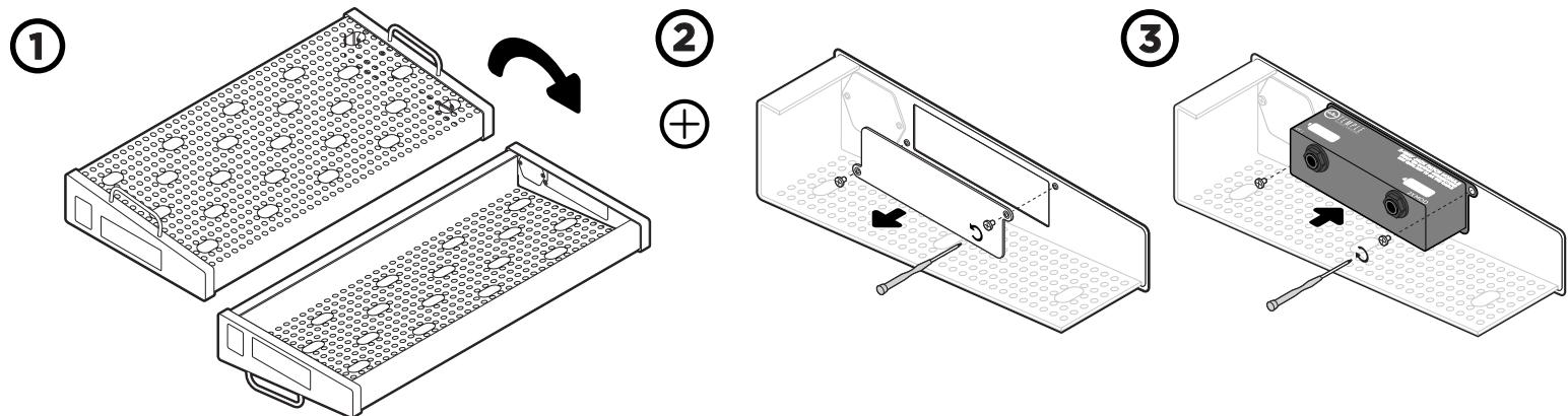
The 2X MOD Pro mounts in the Modular Endpanel of your Templeboard and allows you to route two buffered 1/4" inputs and outputs through the side of your board.
