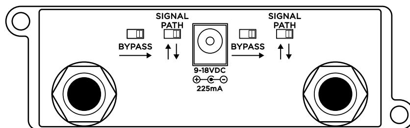
**BYPASS:** Move to the right to disengage the buffer on that channel. Move left to re-engage.
