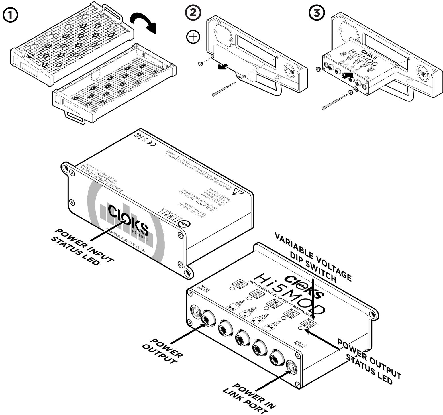
The Hi5 MOD is a high-current, isolated power module. It offers clean power across five outputs that easily integrate into the side of your Templeboard. The variable voltage offers flexibility to cater to most pedals' power requirements.
